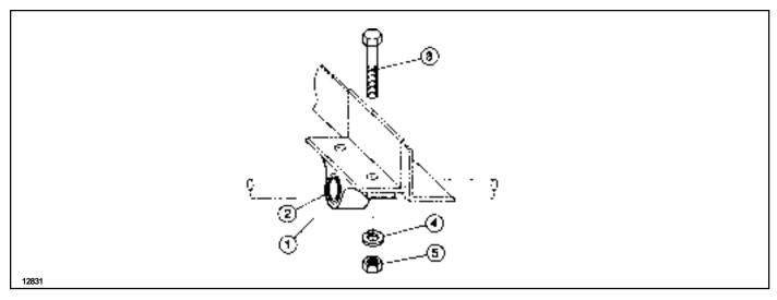
Figure 2. Cross Shaft Bearing Assembly. (Catalog Number 904625).
