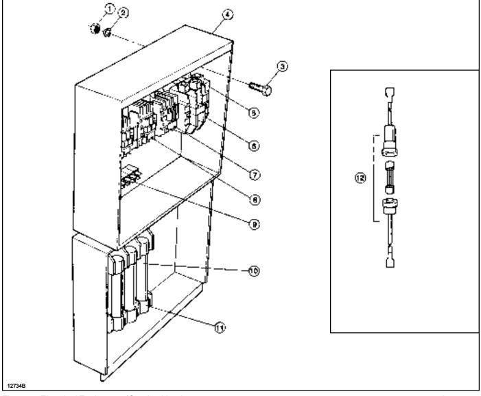
$Figure \, 6. \,\, Electrical \, Enclosure. \,\, (Catalog \, Numbers \, 905385, 905386, 905387, 905397, 905398, 905399, 913155 \, thru \, 913158 \, and \, 913165 \, thru \, 913169).$
