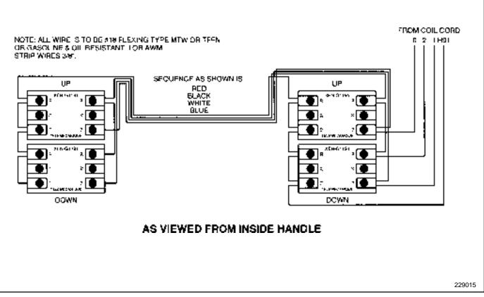
Contact Block and Jumper Assembly.
