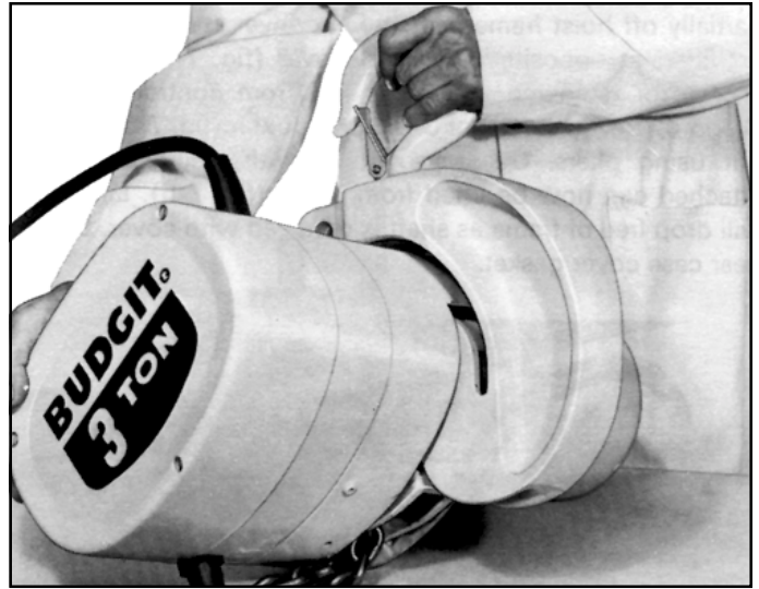
Figure 7-3. Removing 3 Ton Hanger Bracket from Hoist Frame
