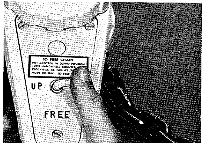
Figure 2-2. Placing Finger-Tip Lever in "DN" Position
