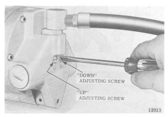
Figure 2-4. Hoisting and Lowering Speed Adjustment.
