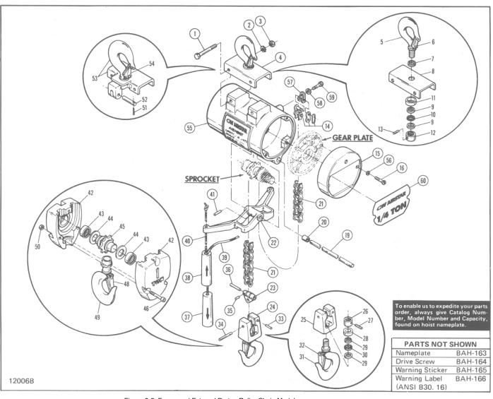
Figure 8-2. Frame and External Parts - Roller Chain Models.
