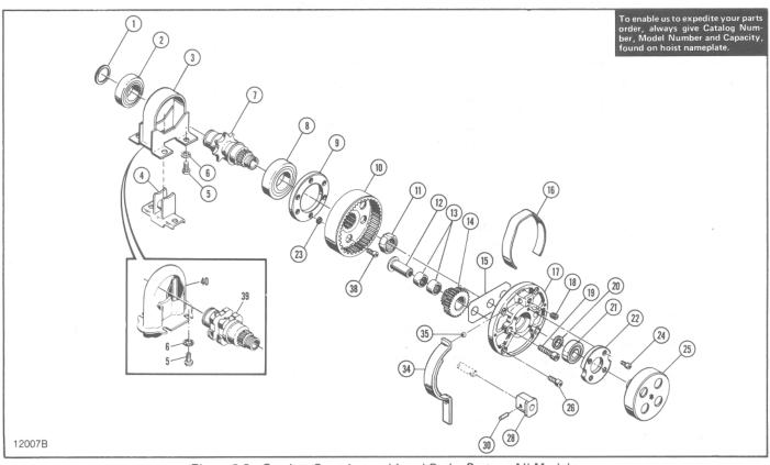
Figure 8-3. Gearing, Sprocket and Load Brake Parts – All Models.
