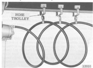
Figure 2-2. Air Hoist Supported by CM Hose Trolleys.
