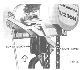
Figure 3-3. Control Lever Being Tripped by Lower Block.
