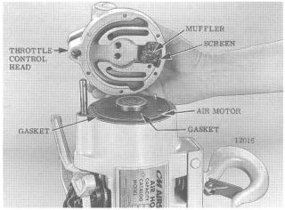
Figure 7-6. Removing Control Head Assembly.
