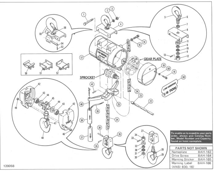
Figure 8-1 . Frame and External Parts - Coil Chain Models.
