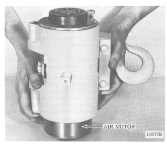
Figure 7-7. Removing Motor from Frame.
