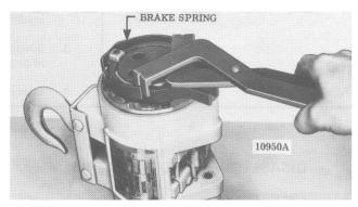
Figure 7-5. Removing Brake Spring Using Special Tool.
