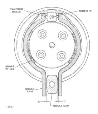
Figure 7-15. Brake Adjustments.
