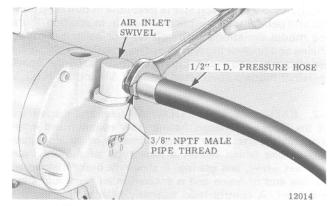
Figure 2-1. Connecting Air Hose to Hoist.
