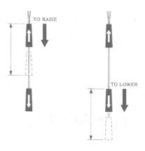
Figure 3-1. Pull Cord Control Handles.
