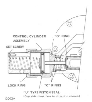
Figure 7-14. Section View Showing Assembly of Control Cylinder on Control Head (Pendant Throttle Control Models).
