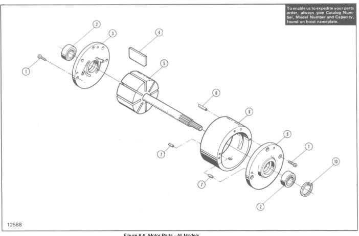
Figure 8-5. Motor Parts - All Models.
