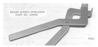
Figure 7-4. Special Tool for Removing Brake Spring.
