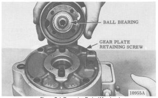
Figure 7-J. Removing Brake Wheel and Ball Bearing Assembly.
