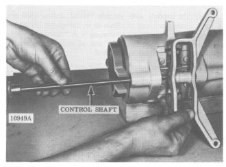
Figure 7-3. Removing Control Shaft.
