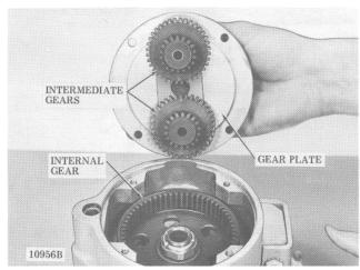
Figure 7-10. Removing Gear Plate and Intermediate Gears.
