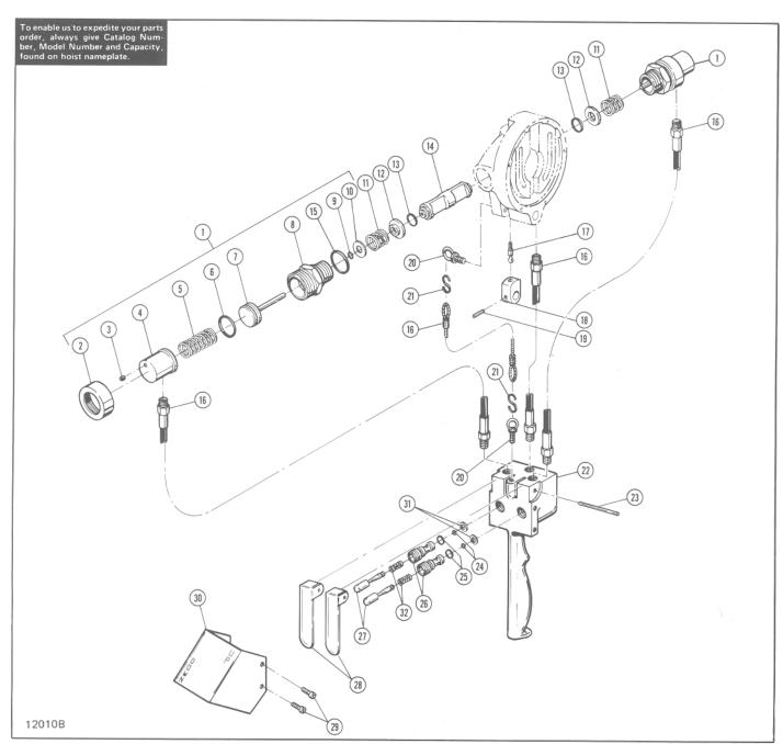
Figure 8-6. Control Cylinder and Pendant Throttle Control Parts.
