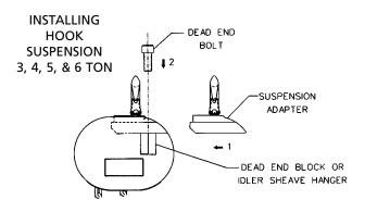
If the hook is to be perpendicular to long axis of hoist per step b above, rotate the hook to that position and firmly tighten the keeper plate screw while making sure the loose pin engages the slot in keeper plate.
