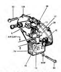
Figure 1. Motor Brake Adjustment
