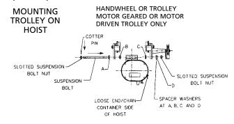
3. For 2 ton units, assemble a slotted nut to one end of each suspension bolt and secure it using a cotter pin. Spread legs of cotter pin to keep it in place. Using Table 2 as a reference for washer spacing, assemble side frames and bolts and washers together as shown below. Do not install remaining cotter pins at this time. These are to be installed after the trolley is mounted on the beam.
