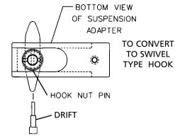
b. If it is necessary to position the hook so that the plane of the hook is perpendicular to the long axis of hoist, first convert to a swivel type hook as described above. Rotate the hook 90 degrees and slide the loose pin (packed with the suspension) through the hole in the side of the suspension adapter and engage the hole in the hook nut.
