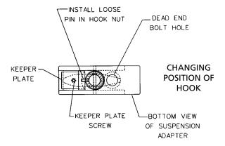
c. Slide the suspension adapter into cavity on top of hoist. Install dead end bolt and thread it by hand to engage the dead end block (3, 4 and 5 ton double reeved units) or idler sheave hanger (5 and 6 ton units). Then tighten dead end bolt to a seating torque of 120 pound feet (160NM).
