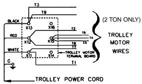
TROLLEY VOLTAGE CONVERSION (Connections shown are for 208-240 volt operation)
