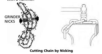
2. Use a 7 inch (177 mm) minimum diameter by 1/8 inch (3.1 mm) thick abrasive wheel (or type recommended by wheel supplier) that will clear adjacent links
