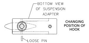
c. After the hook is in the desired position, slide the suspension adapter into cavity on top of hoist and secure it using the suspension adapter screw from the kit. Tighten screw to a seating torque of 16 pound feet (22 NM).
