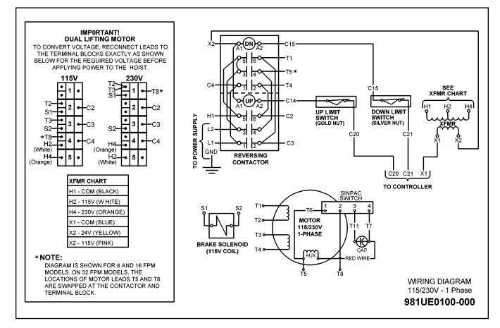
Figure 7A — Wiring Diagram for 115/230V - 1 Phase Models
