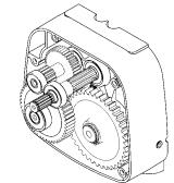
**Figure 6 - Assembled Gearing**
