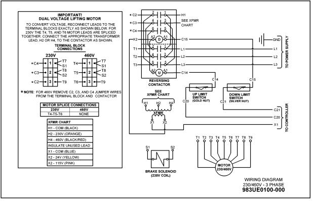
Figure 7B — Wiring Diagram for 230/460V - 3 Phase Models
