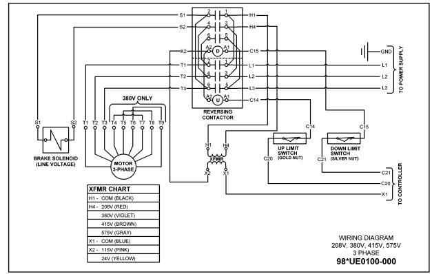
Figure 7C - Wiring Diagram for 208V, 380V, 415V and 575V - 3 Phase Models \*Factory supplied wiring diagrams will have numbers beginning with 985 for 575V, 987 for 208V, 988 for 380V and 989 for 415V.
