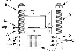
Figure 4 — Brake Assembly
