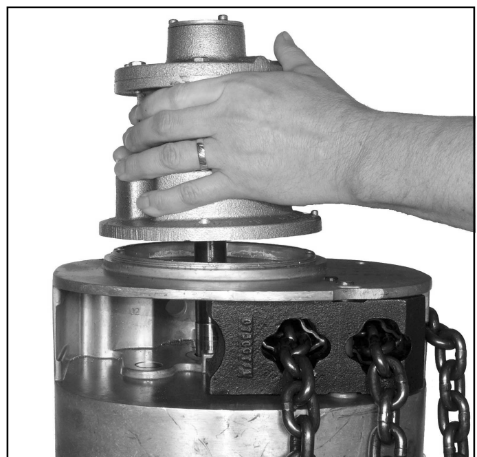
Figure 7-8. Removing Motor Assembly
