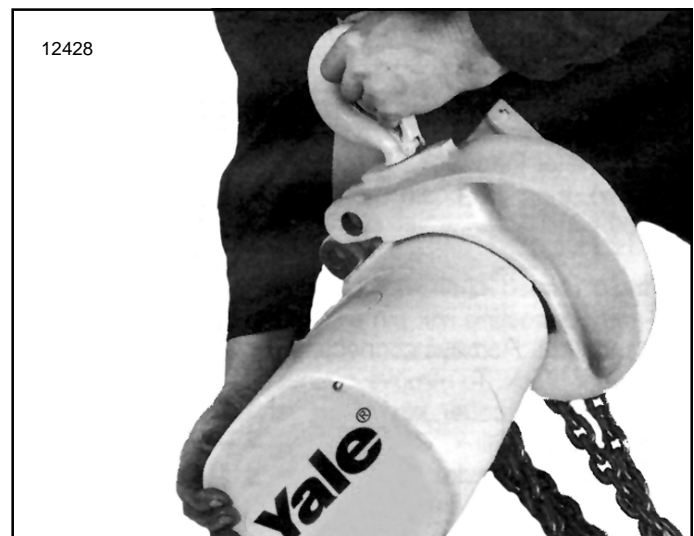
Figure 7-2. Removing 3 Ton Hanger Bracket from Hoist Frame
