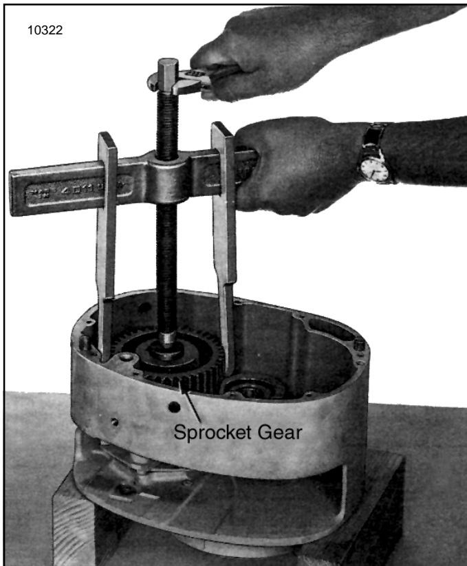
Figure 7-9. Pulling Sprocket Gear from Sprocket Shaft Using Common Puller
