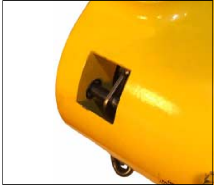
Figure 7-12. Removing Chain Guide Support Pins
