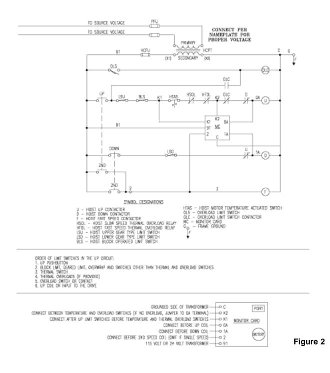
**Warning:** The Pulse monitor card is electronic equipment that requires earth ground to reduce potential for false data. If a dedicated ground is not available, make sure reference ground to all control transformers have one common point.
