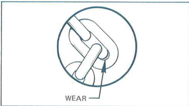
Figure 5-1. Check Chain Wear at Bearing Surfaces Between Links.
