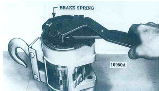
Figure 7-5. Removing Brake Spring Using Special Tool.
