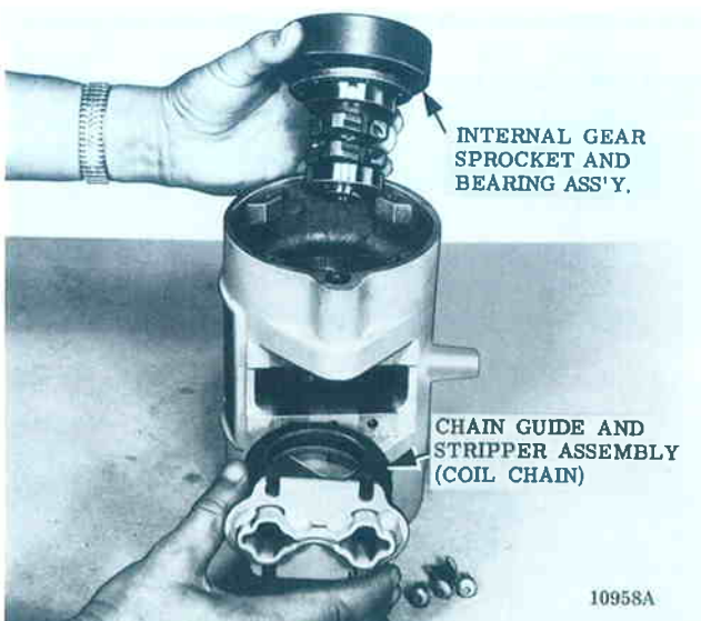
Figure 7-12. Removing Internal Gear, Chain Sprocket and Ball Bearing Assembly (Coil Chain Model).
