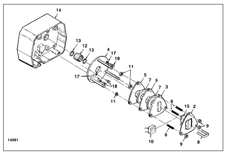
Figure 7-7A. Motor Brake Parts - (2 HP) Models
