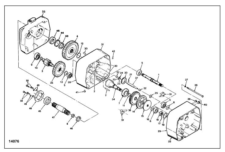
Figure 7-4. Hoist Transmission
