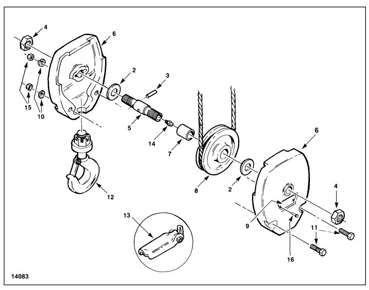
Figure 7-9A. Bottom Block (1 & 2 Ton) S2 Models Only
