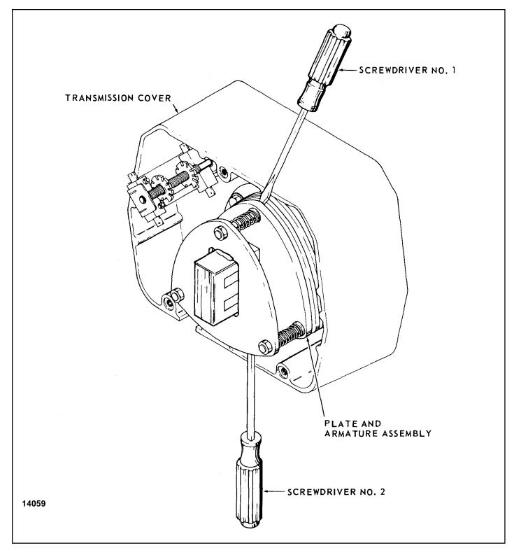
Figure 4-8. Load Brake Function Check
