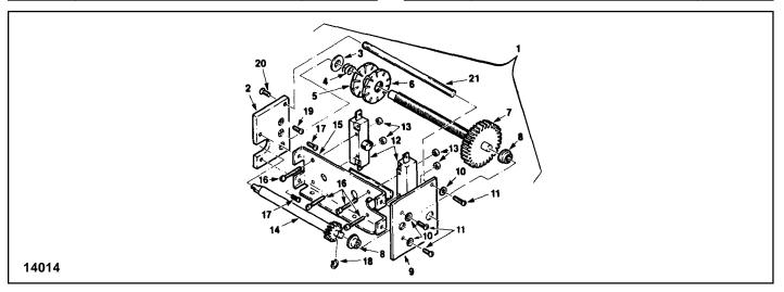
Figure 7-6A. Long Lift Limit Switch 1 & 2 Ton with 70 ft. Lift and 3 Ton with 35 ft. Lift Only
