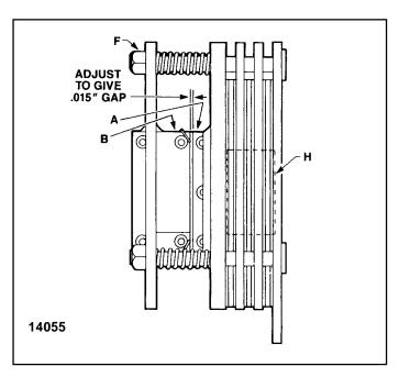
Figure 4-2 Motor Brake Adjustment
