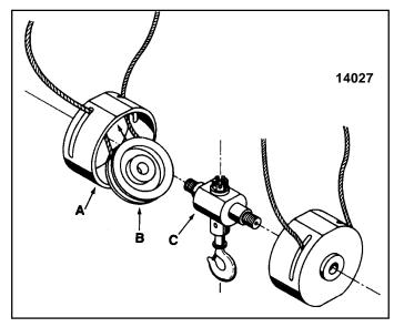
Figure 4-4. Assembly of Load Block D2 & P2 Models
