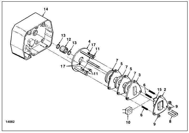
Figure 7-7B. Motor Brake Parts (3 HP) Models
