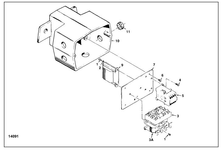
Figure 7-14B. Trolley Control, Two Speed (Two Speed Trolley with One or Two Speed Hoist)
