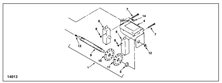
Figure 7-6. Limit Switch Parts
