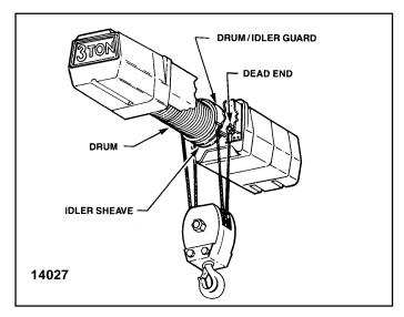
Figure 4-3D. Wire Rope Reeving - 3-Ton, S4 Models
