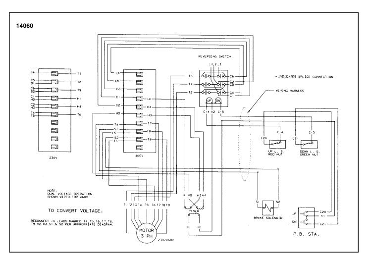
Figure 6-1. Wiring Diagram 230/460V, 3 Phase, Single Speed Hoist 983EC44C
