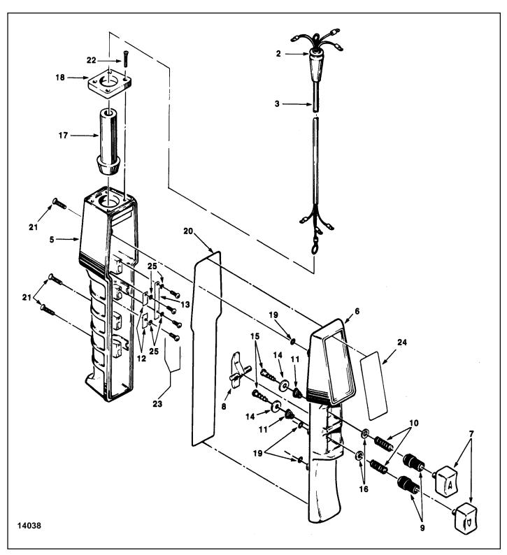
Figure 7-8A. Pushbutton (Single Speed Hoists)
