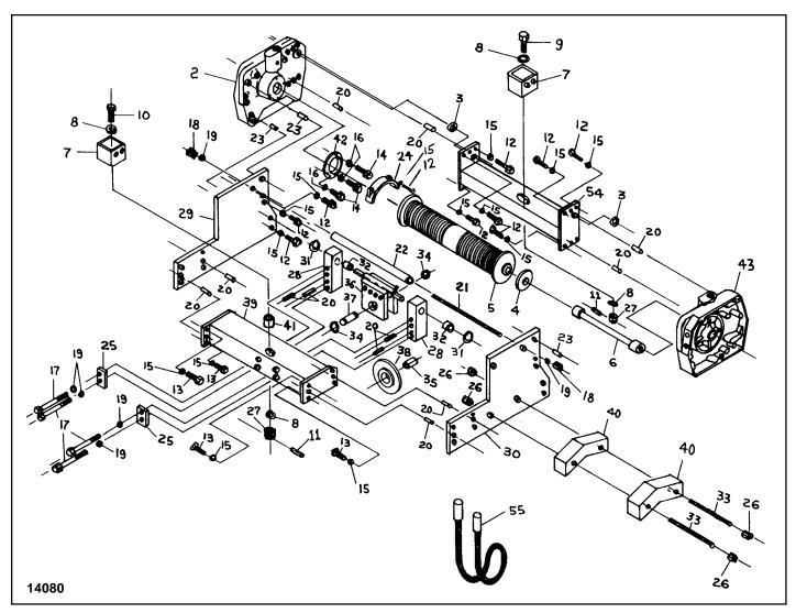
Figure 7-5D. Drum Area (1 & 2 Ton) D2 Models Only
