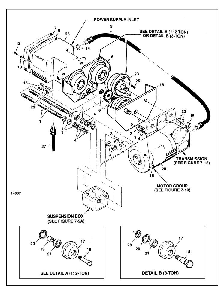
Figure 7-10B. Trolley General Assembly (Single Speed Hoist, Two Speed Trolley, Two Speed Hoist, Single Speed Trolley, Two Speed Trolley)
