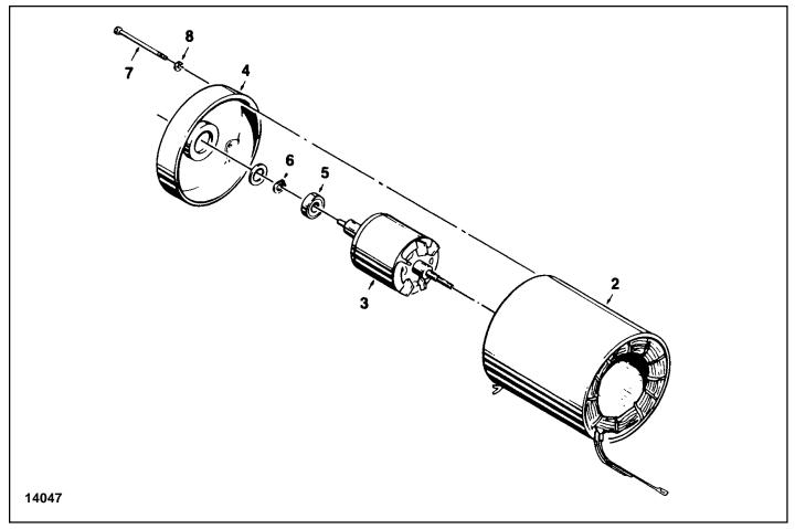
Figure 7-13. Trolley Motor Parts
