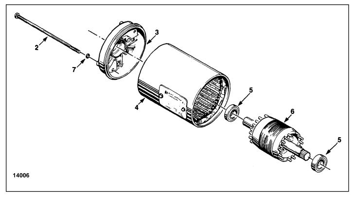
Figure 7-2. Hoist Motor Parts
