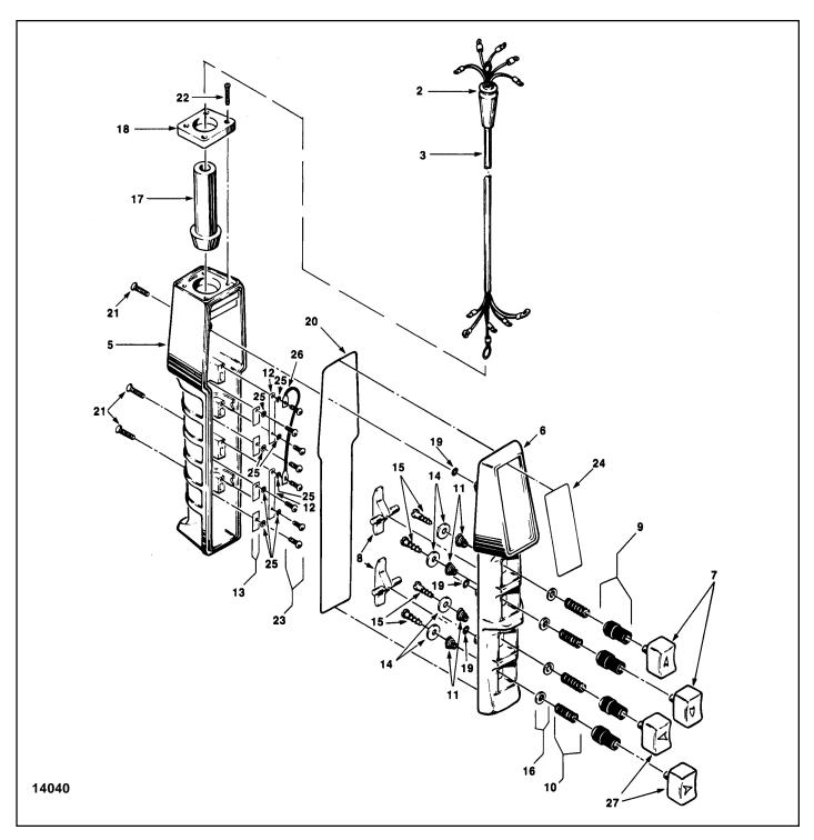
Figure 7-8C. Pushbutton (Single Speed Hoist - Single Speed Trolley)
