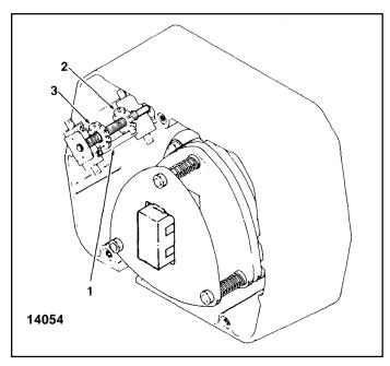
Figure 4-1 Limit Switch Adjustment
