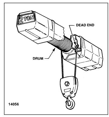
Figure 4-3A Wire Rope Reeving (1 & 2-Ton, S2 Models)
