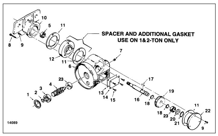
Figure 7-12. Trolley Transmission
