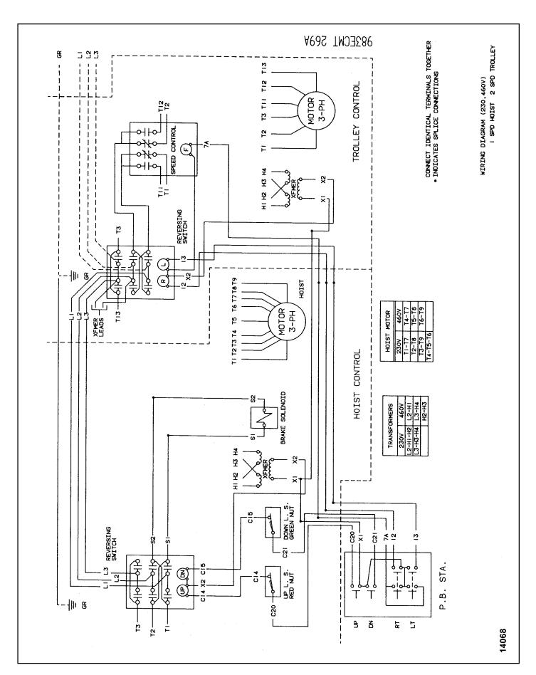
Figure 6-9. Wiring Diagram 230, 460V, 3 Phase, Single Speed Hoist & Two Speed Trolley 983ECMT269A
