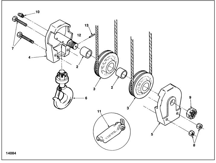
Figure 7-9B. Bottom Block (3 Ton) S4 Models Only
