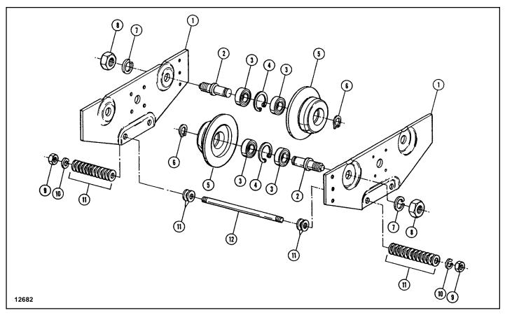
Figure 3. Push Type Rigid Mount Trolley Assembly. (4"  $\varnothing$  Wheels — 3-1/8" & 5" c/c Pins.)
