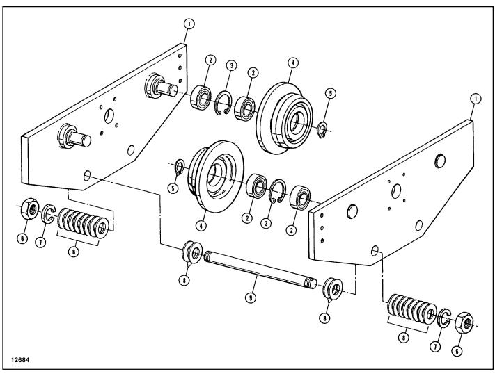
Figure 5. Push Type Rigid Mount Trolley Assembly — (6½" & 8"  $\varnothing$  Wheels) and Trailer Trolley \* - (6½"  $\varnothing$  Wheels).
