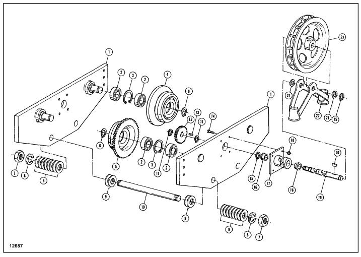
Figure 8. Hand Geared Rigid Mount Trolley Assembly (6½" & 8"  $\varnothing$  Wheels.)
