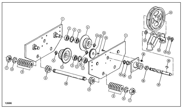
Figure 7. Hand Geared Rigid Mount Trolley Assembly (4"  $\varnothing$  Wheels — 6" c/c Pins.)
